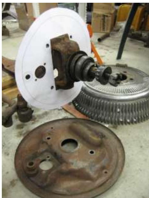
Brake backing plate and drum from 1963 Buick Riviera
